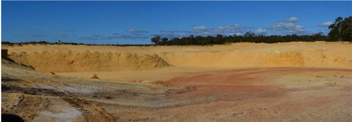
Plate 1 - Panorama of Lot 7 extraction area, top soil scraped from immediate surrounds of active extraction area, vertical depth of extraction approximately 4 metres.
